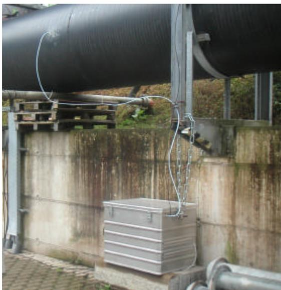
OdourVector has a GSM data modem interface and can be remote controlled.
