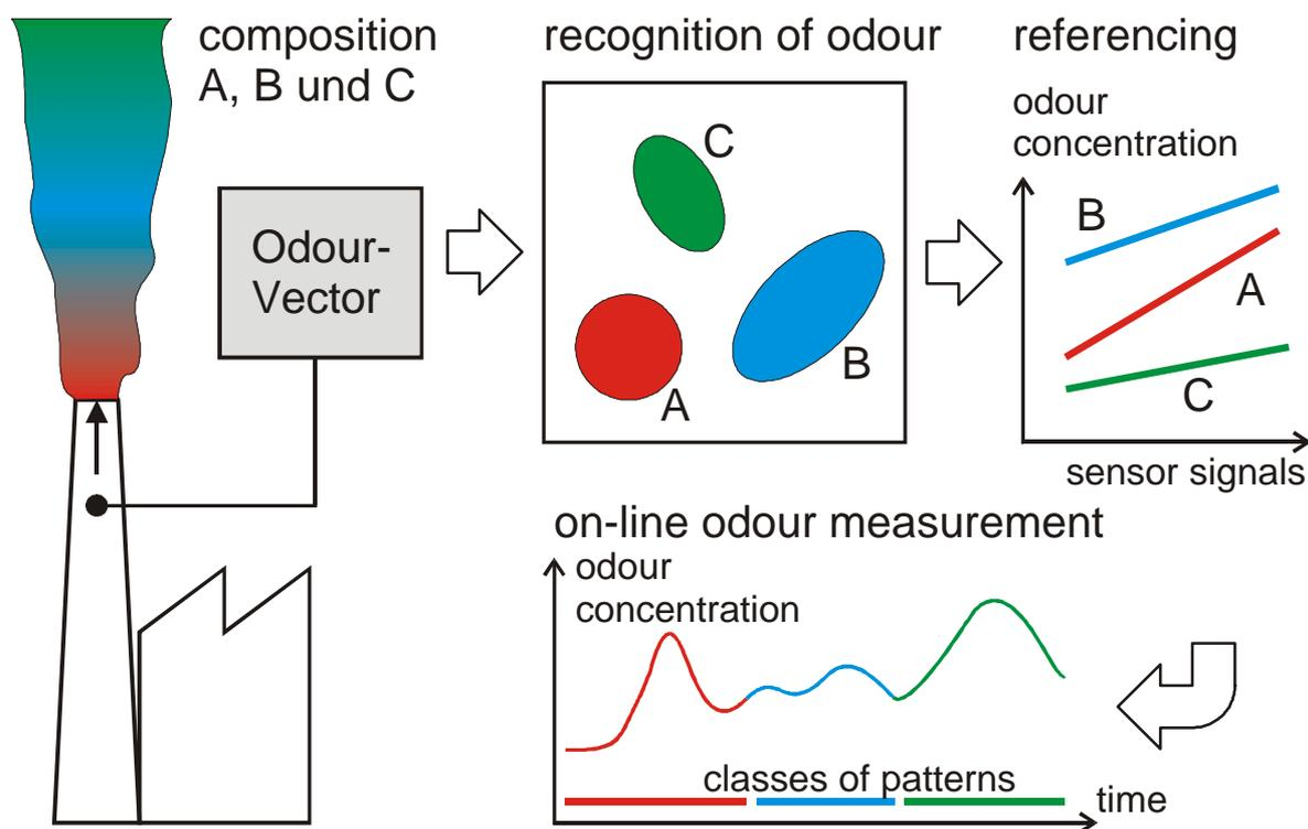
Technical-sensory odour measurement using the measurement system *OdourVector*<sup>TM</sup>.
